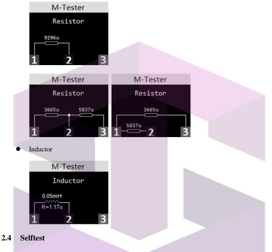
Short all three Probes, short press the multifunction key, the tester will be automatically calibrates itself.
